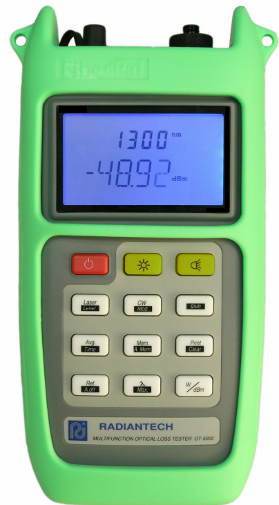
Multifunction Optical Loss Tester (OT-5000)
